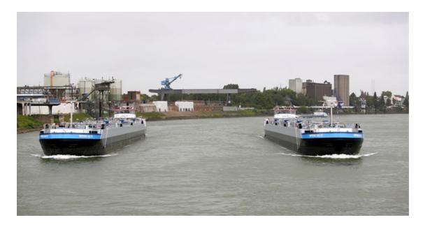
"Gas tankers are a flexible solution for supplying energy and raw materials to industries, and an alternative to transporting liquid gases in pipelines. Gases have to be liquefied before they are transported. The reduction in volume resulting from this enables the vessels to accommodate greater loads. This means that inland waterway vessels have become a very efficient and eco-friendly means of transport," Rossouw says.
