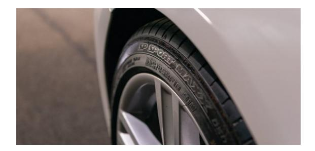
High speed stability is ensured through features such as the wide and solid outer shoulder block, high stiffness blocks for optimum road contact and a high rigidity construction using more than two nylon reinforced layers to minimise tread profile expansion and provide secure road contact at high speed.
