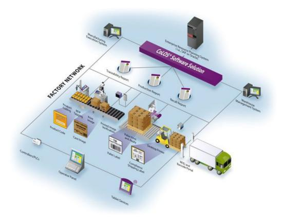
Traditionally, batch and code data is manually entered into the system. However, if a code is incorrectly entered the whole line grinds to a halt while the root of the problem is investigated and rectified. This causes massive delays on the production line and can lead to further complications such as cross-contamination. Centralised data management ensures fast and accurate retrieval of production batch codes because the coding information is automated.
