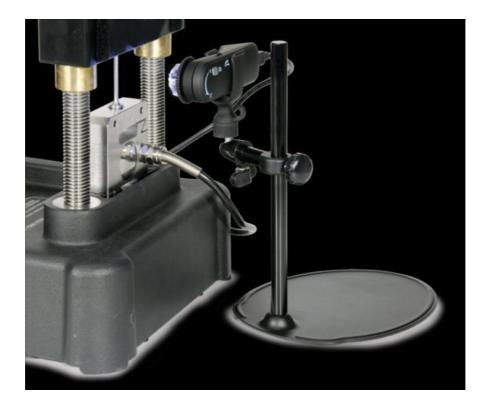
This Microscope Camera includes a stand, built in adjustable LED lighting, and has a 60x Optical Zoom. You can see even the tiniest changes during an experiment (as pictured for stress and strain) or else use it as a working microscope for Life Science activities.
